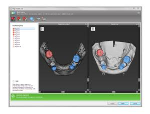
Pairs of corresponding regions should not lie on an (approximately) straight line and must be set at anatomically significant positions and as far away from each other as possible.
